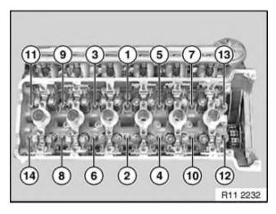
Release cylinder head bolts from outside to inside in sequence 14 to 1.
