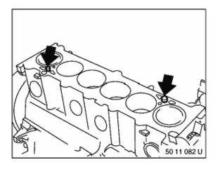
Check dowel sleeves for damage and correct installation position.
