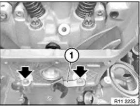
Install cable holder (1) and screws.
