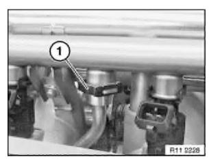
Detach retaining clip (1) of fuel feed line.
