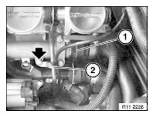
Unlock water hose (1) and detach from return line. Release upper screw of fuel feed line (2) from return line.
