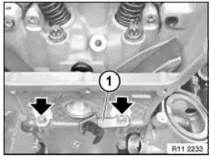
Release screws between cylinder head and timing case cover. Remove cable holder (1).
