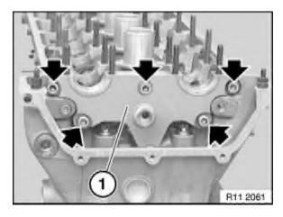
Install thrust bearing flange (1). Install and tighten down screws.
