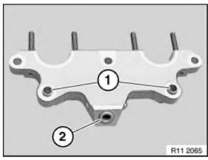
Check dowel sleeves (1) for damage and correct installation position.
