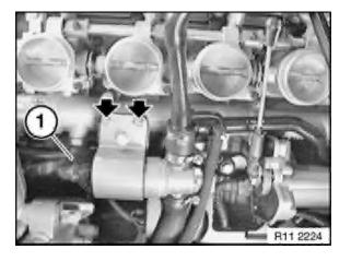
Detach bracket for idle-speed control valve from return line and lay with hoses to one side.
