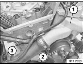
Replace O-ring on pipe (3). Install pipe (3). Install belt pulley (2).
