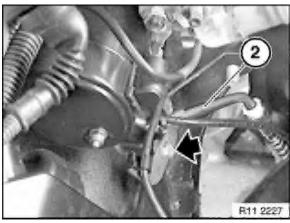
Release lower screw of fuel feed line (2) from engine block.
