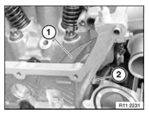
Replace sealing washer for screw (2). Screw down sliding rail (1) with screw (2).
